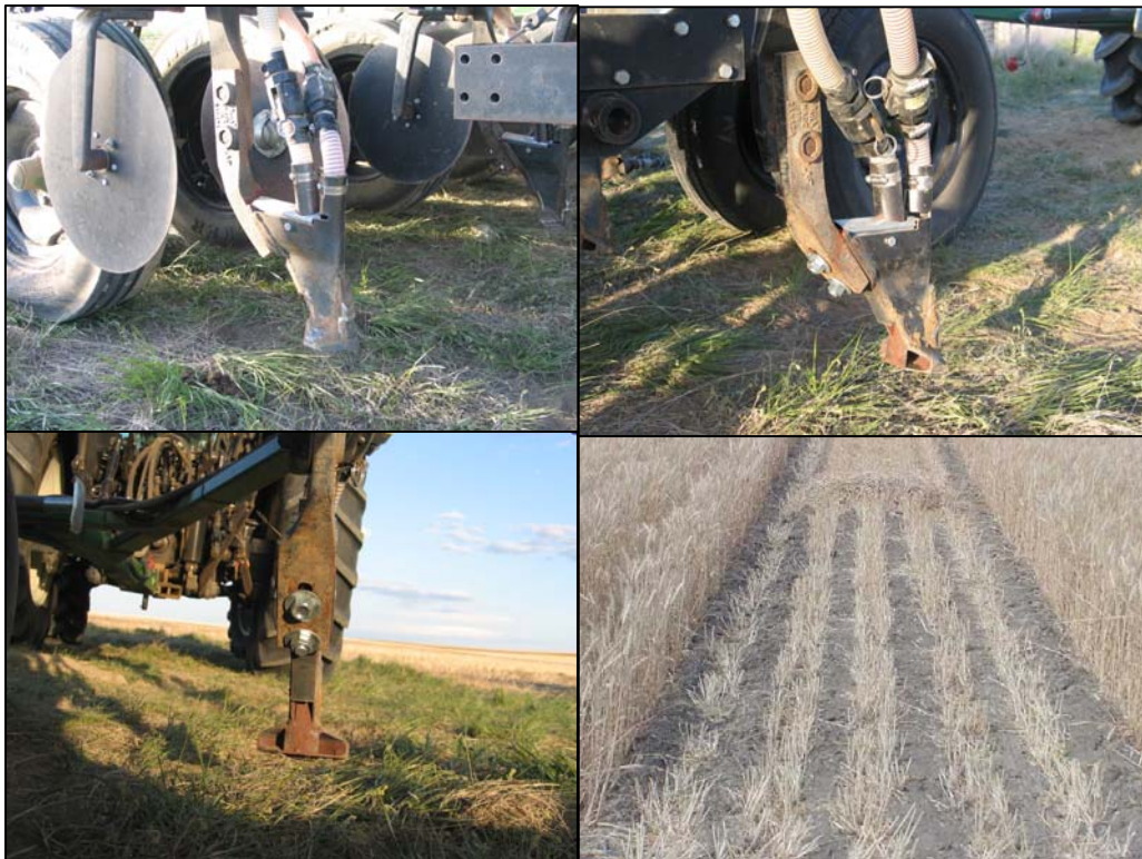
Figure 2. ATOM JET Paired Row (Paired-Separate, Seed Band Width = 6.0 Inches)
