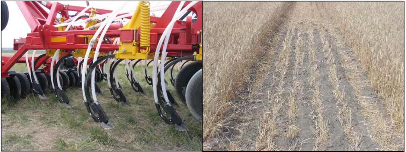
Figure 19. DUTCH Low Draft Dbl-Shoot: 0-0-0 w/Seed+70-40-0 via FertBand (Paired/Joined, Band Width = 4.9 Inches)
