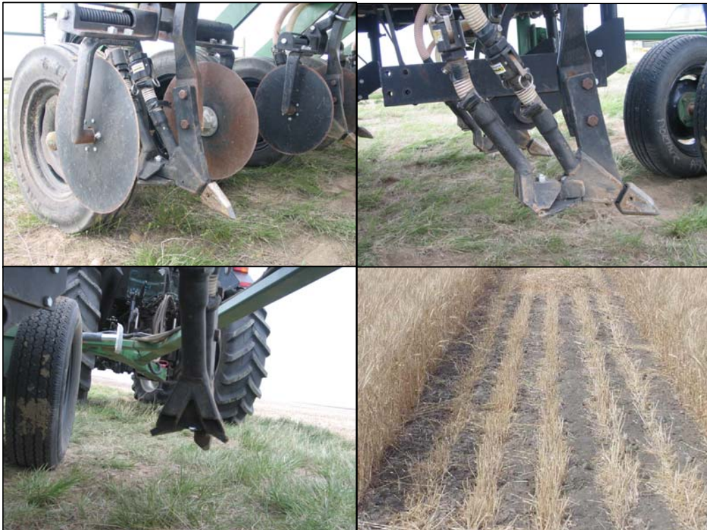
Figure 4. DUTCH 3.5" Paired Row (Solid, Seed Band Width = 4.9 Inches)
