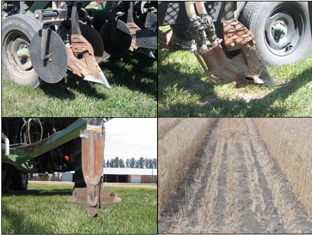
Figure 11. GEN 200 T2x2 Paired Row (Paired/Separate, Seed Band Width = 6.8 Inches)
