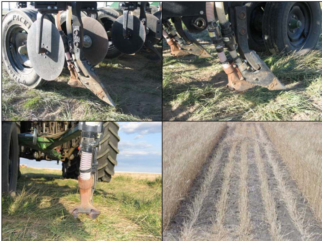
Figure 10. FLEXICOIL Stealth w/ Paired Row Attachment (Solid, Seed Band Width = 3.9 Inches)
