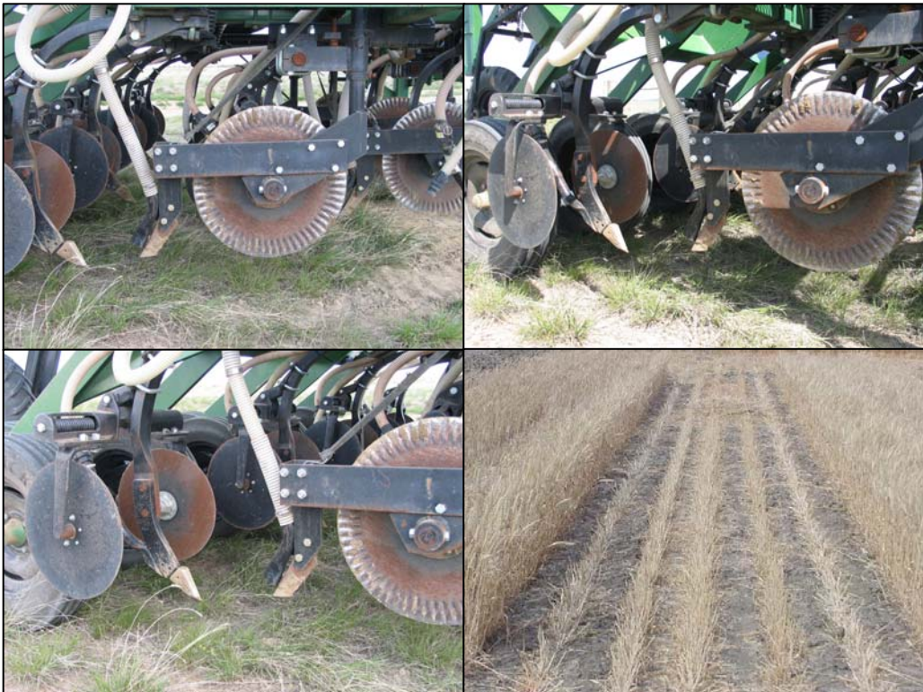
Figure 6. DUTCH SE w/ FARMLAND Mid Banders (Solid, Seed Band Width = 2.6 Inches)
