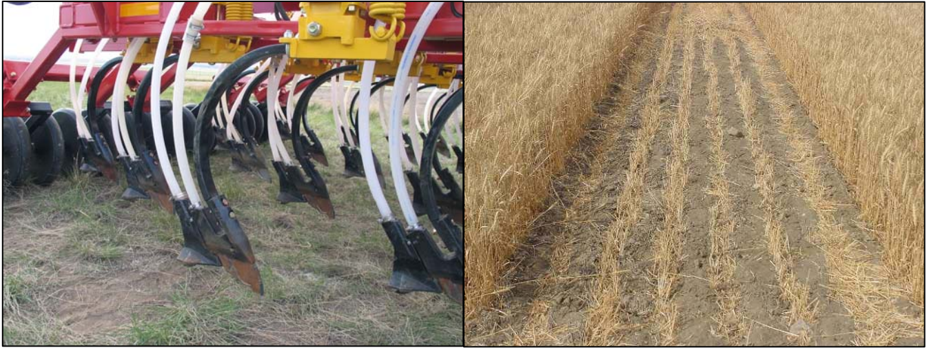
Figure 17. BOURGAULT Dbl-Shoot: 0-0-0 w/Seed+70-40-0 via FertBand (Solid, Seed Band Width = 4.5 Inches)
