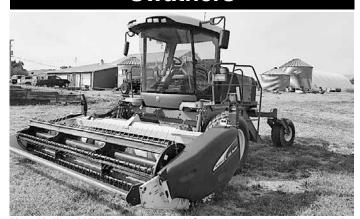
New Holland HW325 swather, 14HS header, new conditioning rolls,
