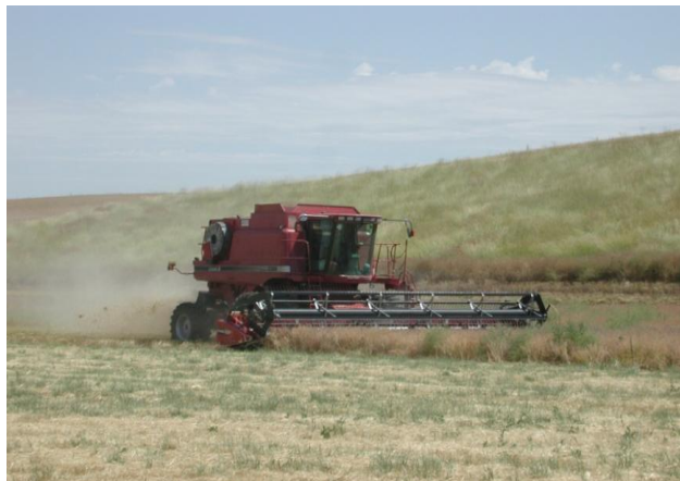
Camelina matures well on the stem. No major adjustments are needed to direct combine the seed. It is important to note that the amount of residue left on the field is less than a comparable wheat crop.
