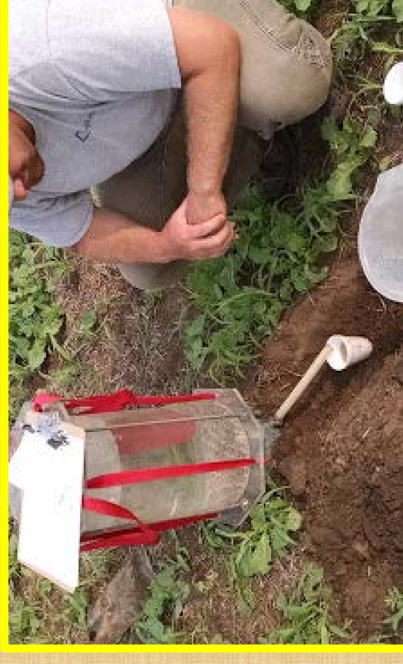
Figure 6. Cornell Infiltrometer being used to sample infiltration rates in different disturbance areas and between rotations.
