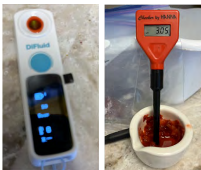
Photo 8. Brix and pH value recorded using DiFluid pocket refractometer and Checker portable pH. Photo by Rojee.
