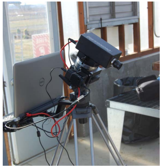
Figure 2. Hyperspectral Imaging System collecting a direct sunlight image.
