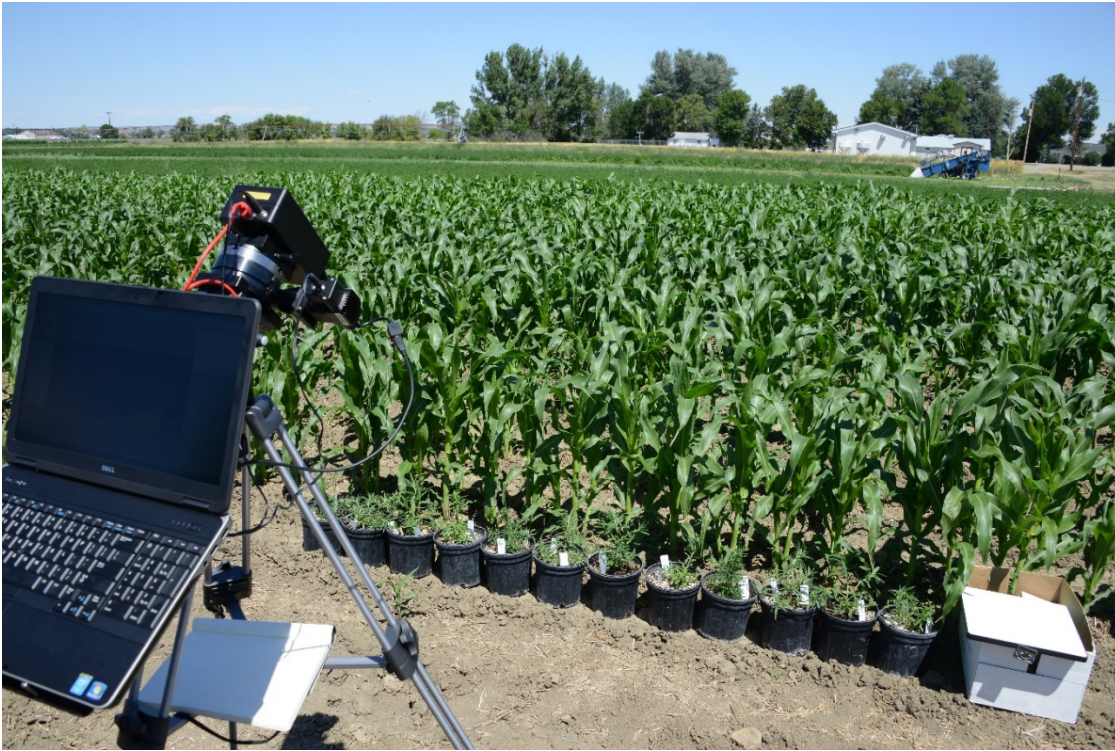
Figure 2. Tripod-mounted hyperspectral imager recording spectral images of potted weeds and crops.
