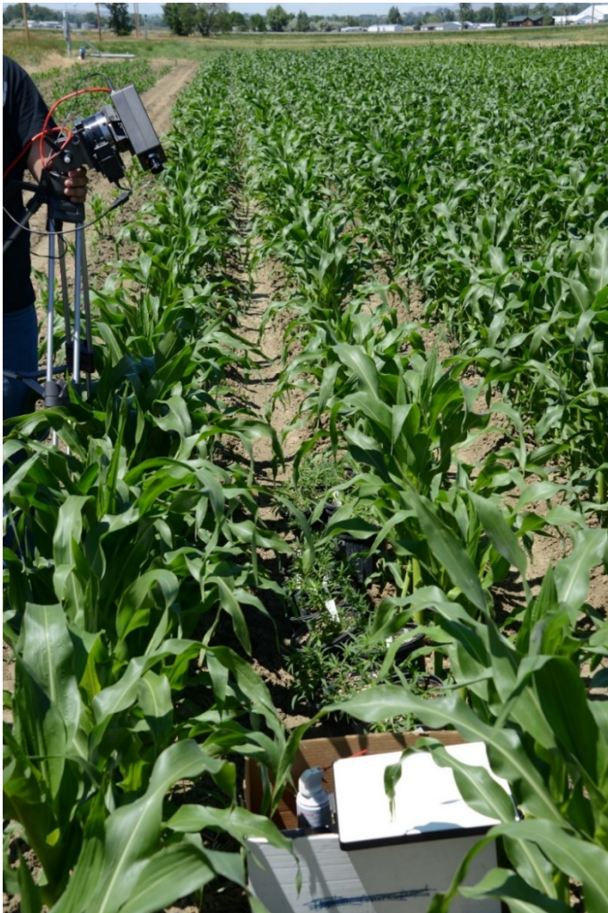
Figure 2. Tripod-mounted hyperspectral imager recording spectral images of potted weeds and crops.
