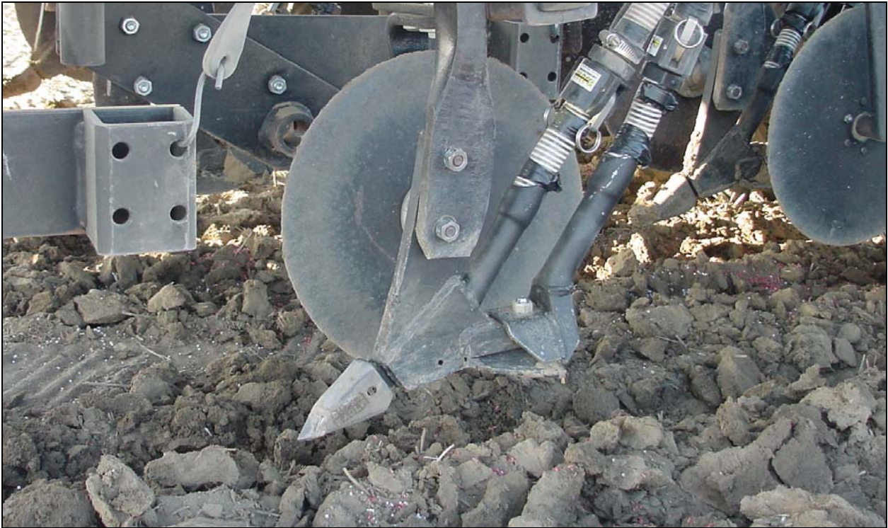
Figure 5a. DUTCH 3.5" Paired Row w/SUPER EAGLE Tip
