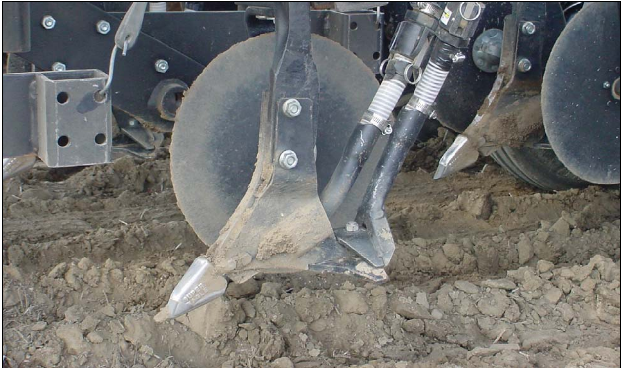
Figure 4a. DUTCH SUPER EAGLE w/5.5" Paired Row Attachment
