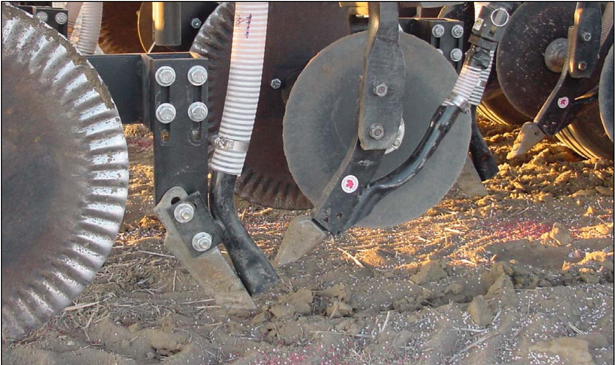
Figure 6a. DUTCH SUPER EAGLE w/FARMLAND Mid-Row Fertilizer Banding Disk
