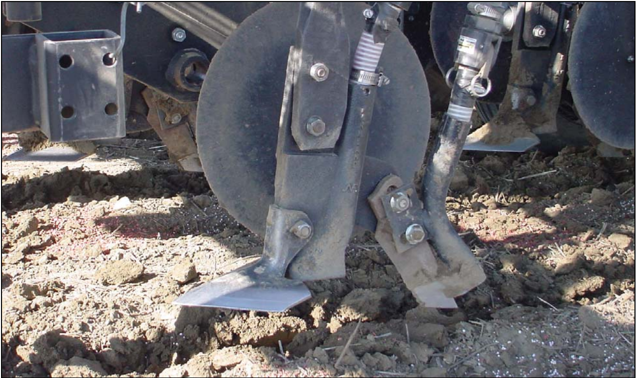
Figure 7a. FARMLAND LOW DISTURBANCE (LD) w/Case-McKay 6" LD Sweep & K3 Backswept Knife
