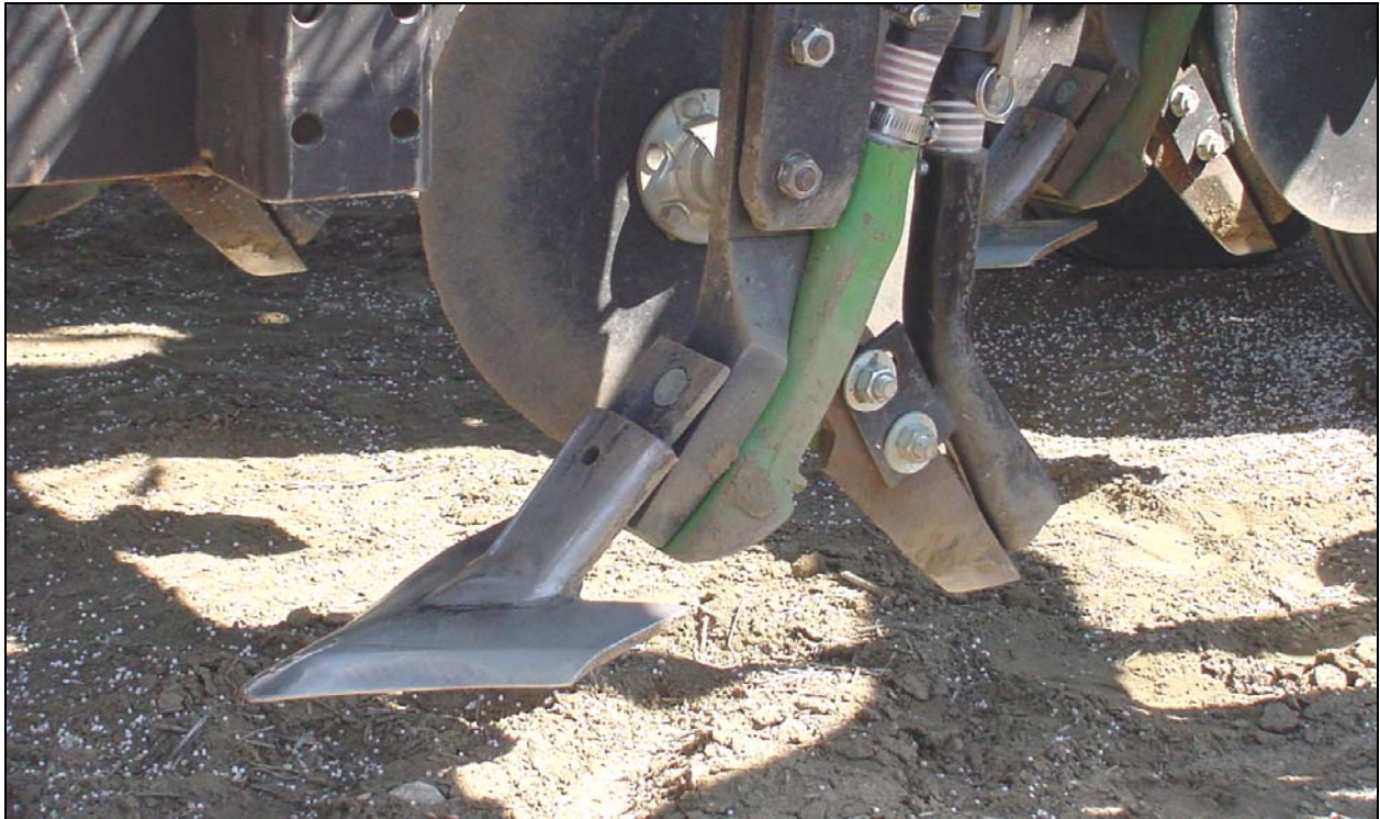
Figure 9a. FARMLAND SB1-SBS1 w/6" Knock-On Sweep & K3 Backswept Knife
