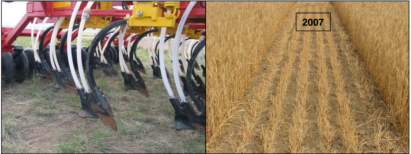
Figure 12. BOURGAULT Dbl-Shoot: 0-40-0 w/Seed+70-0-0 via FertBand (Solid, Seed Band Width = 5.2 Inches)
