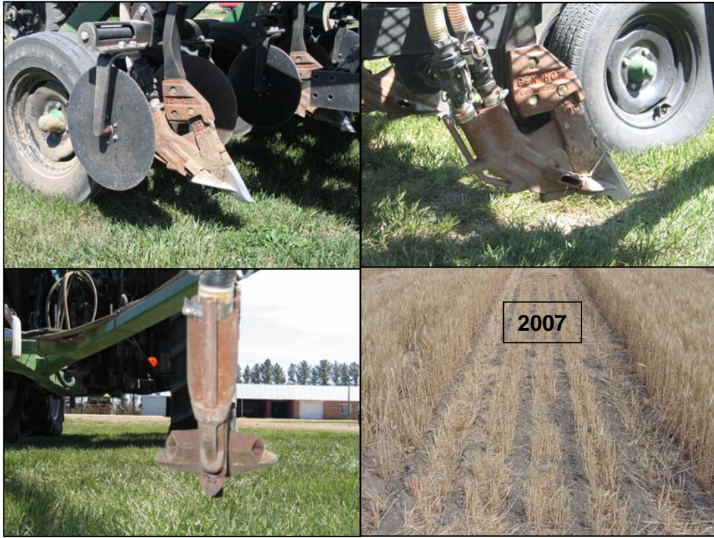
Figure 5. GEN 200 T2x2 Paired Row (Row Style = Paired/Joined, Seed Band Width = 6.7 Inches)
