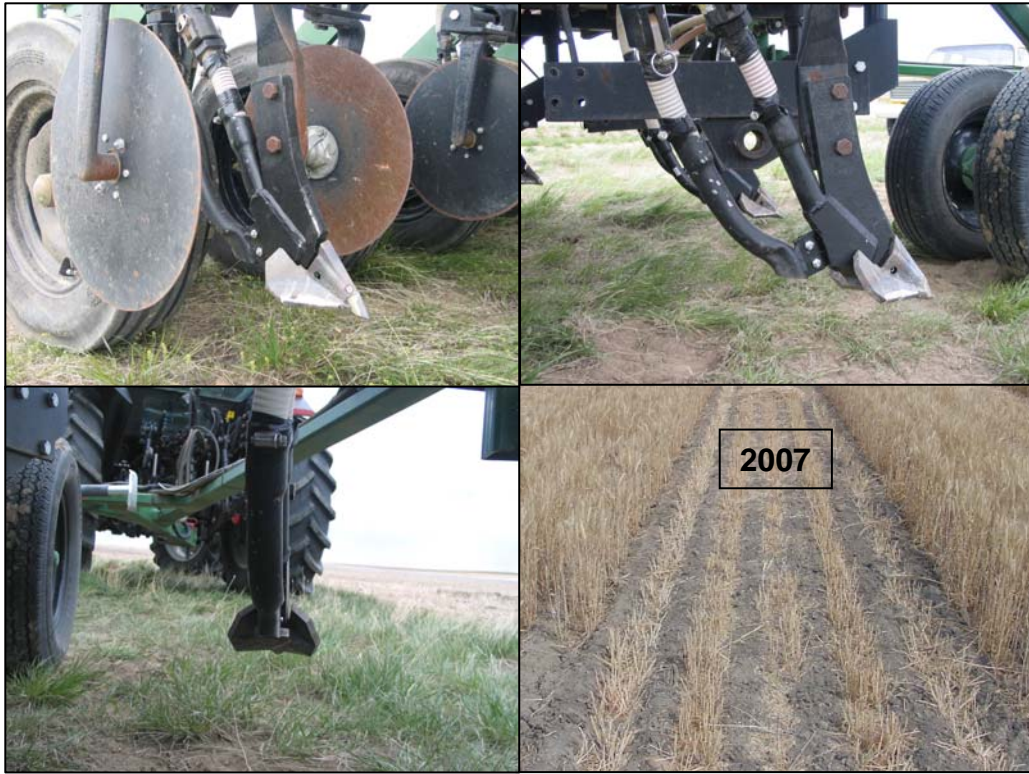
Figure 3. DUTCH Low Draft Paired Row (Row Style = Solid, Seed Band Width = 5.6 Inches)
