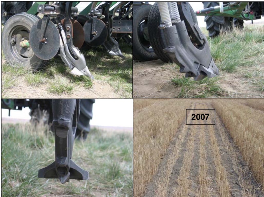
Figure 6. GEN 300 T2 Paired Row (Row Style = Solid, Seed Band Width = 5.8 Inches)
