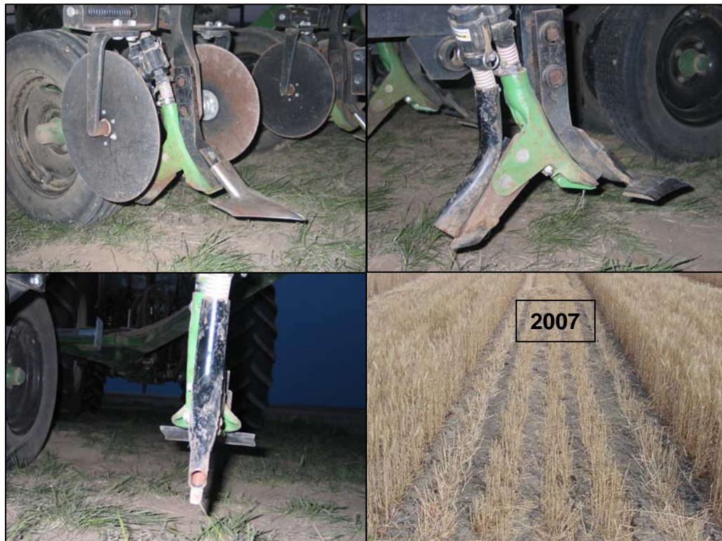
Figure 4. FARMLAND SB1-SBS1 w/ 6" Sweep & Backswept Knife (Solid, Seed Band Width = 6.0 Inches)
