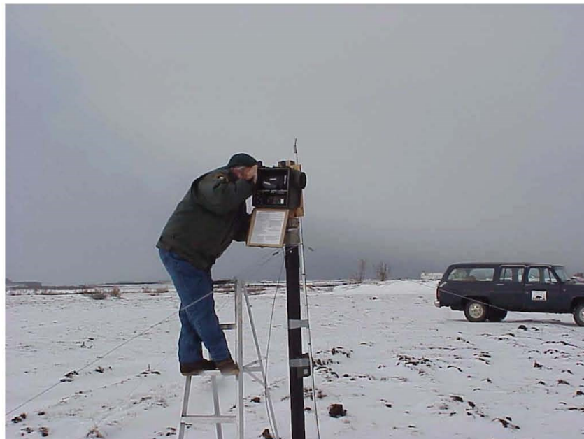
Figure 3. Surveillance camera system mounted approximately 7'-6" above ground level.
