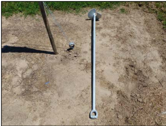
Figure 7. Screw-in, auger-type anchor; 68” long, 3/4” diameter shaft, heavy eye ring and 6” diameter helix screw. Note eye ring sticking out of soil on left. (Photo: Hugh Fraser)
