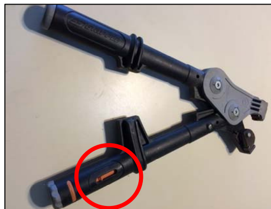
Figure 10. A Torq Tensioning Tool by Gripple TM permits users to set the tension they want by sliding a bar to the desired degree of torq. The tool clicks when the desired tension is reached. (Photo: Leslie Huffman)
