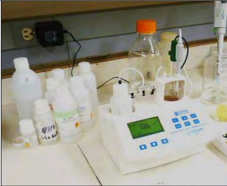
Figure 7. Hanna Instruments Juice Titrator. This equipment makes measure total acidity and pH.
