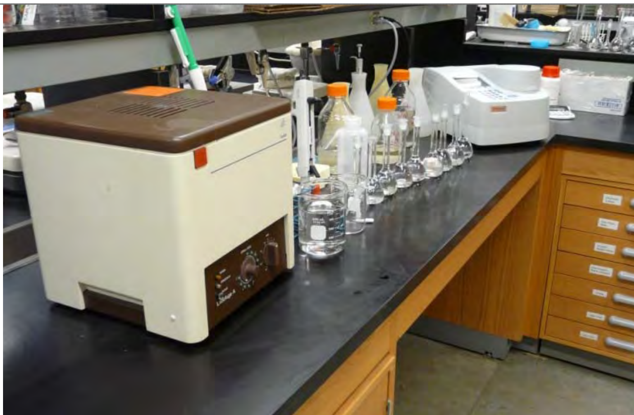
Figure 9. Methyl Cellulose Precipitable (MCP) tannin assay lab equipment The MCP Tannin assay allows us to measure the tannins important for juice and cider quality.
