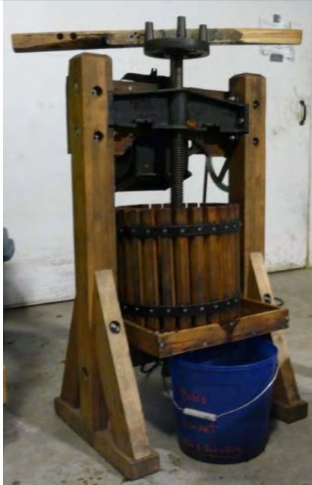
Figure 6. Small scale apple press. This press uses the same basic principles used in larger commercial presses. Ground apples are loaded into a pressing bag which is in turn loaded into the wooden slatted tub. A screw assembly and plate presses the bag of ground apples. The juice is forced through the bag, between the slats of the tub, and into a collection base which drains into a bucket. Attempting to press too much ground apple at once reduces pressing efficiency.
