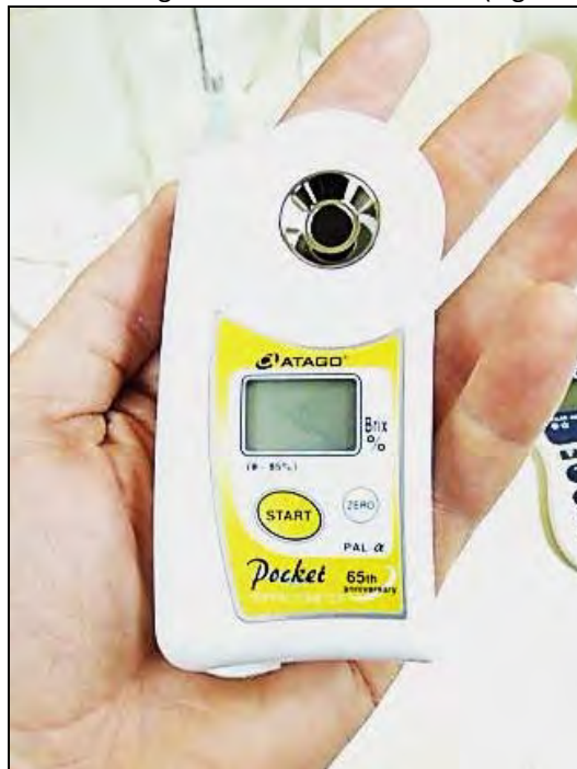
Figure 8. A digital Pocket Refractometer was used to measure the soluble solids of juice. Soluble solids are most made up of sugars. Refractometers have been widely used for decades to measure sugar levels in the food industry.
