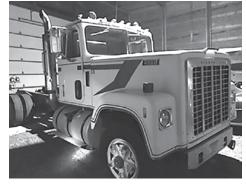
350 Cummins, Jake brake, air brakes, PS, AC, Big Cam engine, Hendrix susp., new bushings. 11x22.5 radials. Lowboy hoist 4000 series - power up and down, auxiliary drill filler. Clean truck, runs excellently.
