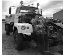
4X4, "V" plow in front, new rebuilt 350 Cummins (never run). Complete with snow plow and new clutch assemblies
