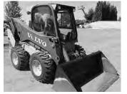
2012 Volvo MC115C 620 hours, enclosed cab with heat and air conditioning, 76" bucket, quick coupler, auxiliary hydraulics, ride control, 2-speed travel, creep speed, good tires, 74 hp, 2600 pound operating load, 5300 pound tipping
