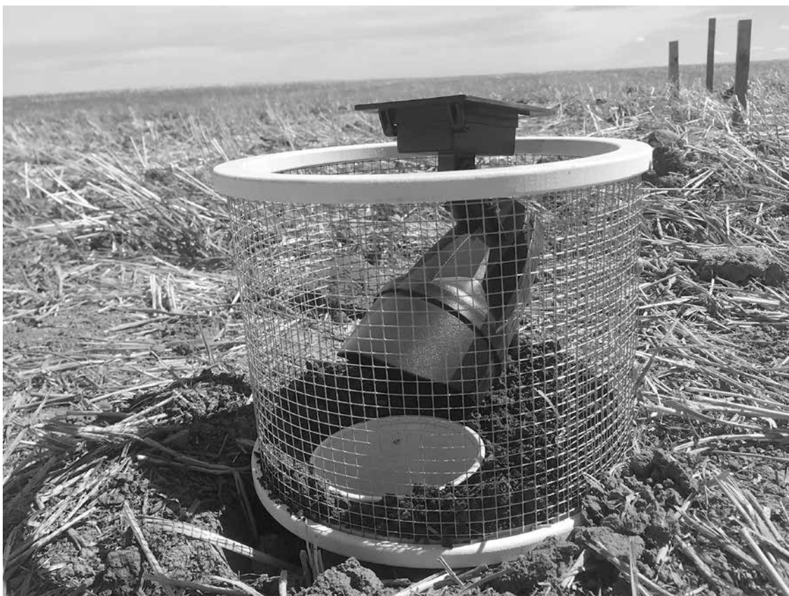
The Noronha Elaterid Light Trap (NELT) that attracts click beetles in fields.
