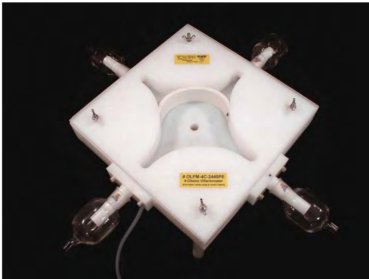
Figure 4. Olfactometer with decision chamber and collection ports installed. Air leaves through the hole in the center and is pumped in through the collection ports. The test insect follows attractants to their source and is collected in the glass collection chamber.
