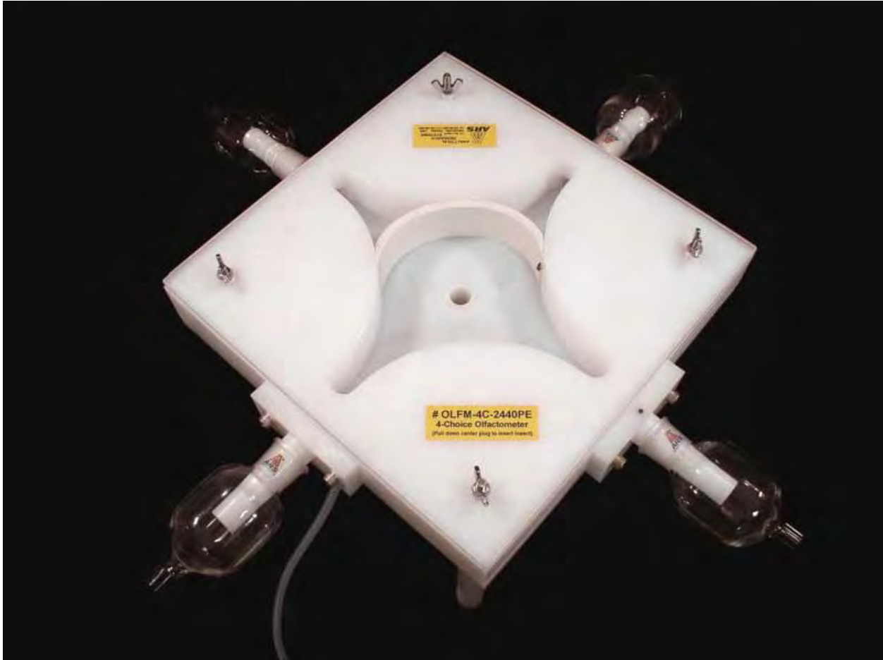
Figure 2. Olfactometer with decision chamber and collection ports installed. Air leaves through the hole in the center and is pumped in through the collection ports. The test insect follows attractants to their source and is collected in the glass collection chamber.
